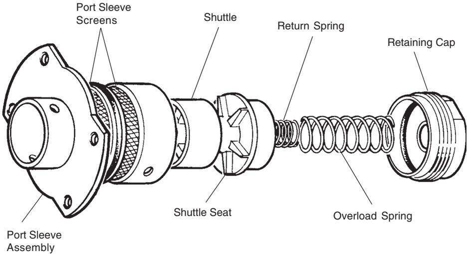
**Shuttle and Sleeve Assembly (Disassembled)**
