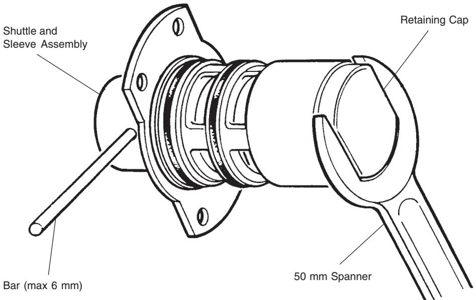
**Shuttle and Sleeve Assembly (Assembled)**
